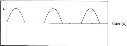
From the CRO, I saw that only the positive AC voltage of the cycle was shown on the screen, hence, the voltage-time graph (above) has no negative voltage.
