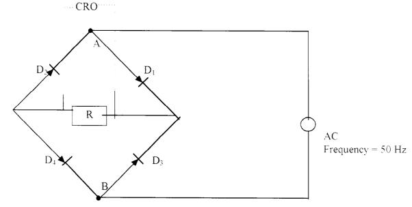
At the instant when "A" is positive, the current flow is through  $D_1$ , the load, and then through  $D_4$ , returning to "B". Diodes  $D_2$  and  $D_3$  are biased-off (non-conducting) and have the full AC voltage across them. On the next half-cycle, when "B" is instantaneously positive, the current flow is from "B", through  $D_3$ , the load, and  $D_2$  to A. Diodes  $D_1$  and  $D_4$  are biased-off.
