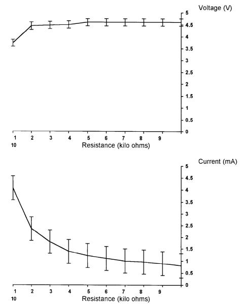
As seen in the graphs above, as the resistance decreases, the voltage decreases and the current increases. The power supply generates voltage E (electro-motive force) that has internal resistance r (constant). When a load resistance is connected to the external circuit, there is a potential voltage  $V_R$  across the resistance R and a voltage drop  $V_r$  across the internal resistance of the power supply.
