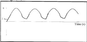
The waveform using full wave rectification is much smoother than the waveform of half wave rectification.
