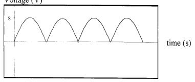
From the CRO, I saw that not only was the positive AC voltage of the cycle shown on the screen but the original negative voltage was now positive, hence, again the voltage-time graph (above) has no negative voltage, but has twice the average voltage than the half rectified wave form, therefore, double the power. Because t = RC, by keeping the resistance a constant at 240  $\Omega$ , I added a capacitor. I observed the effect the capacitor had on the waveform viewed on the CRO.
