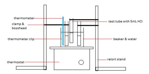
3. The thermostat was set at temperature level 2 and the water was allowed to heat up.
